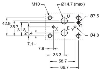
**NOTE:** the positions of the X and Y ports are reversed from the requirements of the ISO Standard
