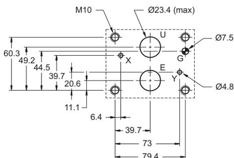
**NOTE:** the positions of the X and Y ports are reversed from the requirements of the ISO Standard
