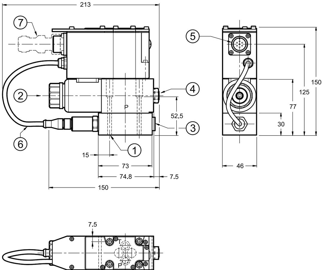
**NOTE:** at the first start up, or after a long period of no use, it is necessary to vent the air through the breather (2) placed at the end of the solenoid tube.
